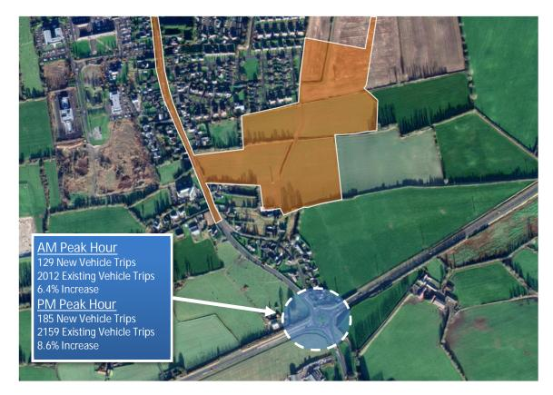
Figure 5.5: Increase in Vehicle Trips Generated Through Key Of-Site Junction (2038
